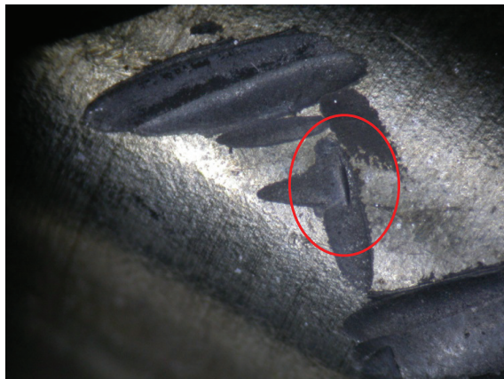
Photo 5 – Fracture within braid wear. 20x
