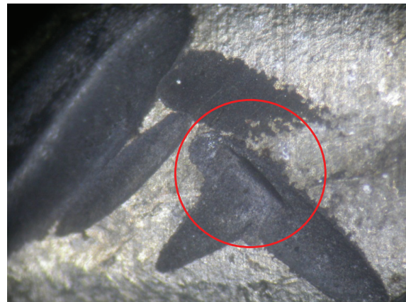
Photo 6 – Fracture within braid wear. 40x
